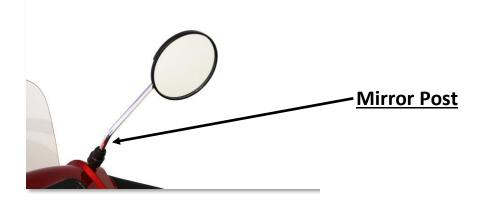
To attach the mirror simply place each mirror threaded end into the mirror post. Turn mirror clockwise and fasten mirror to scooter. Secure using a 14mm wrench on the mirror securing nut.
